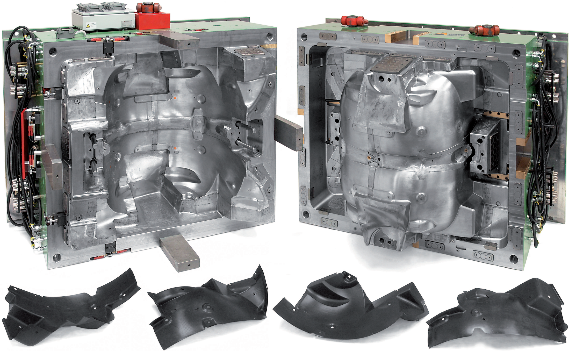
Wheel arches for Renault Master - 29 t - 2180 x 1460 x 1200 mm
